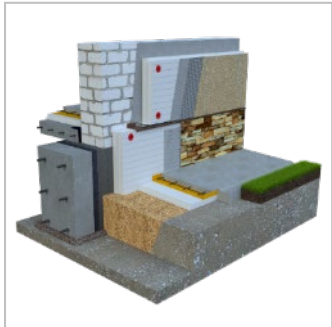
Fastening XPS to waterproofing
