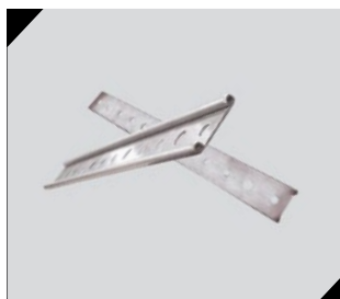
Fastening bars – made from aluminium and magnesium alloy are used to fix waterproofing membrane when changing angles between horizontal and vertical welds and when finishing at the top of the upstand. This can be used to replace the termination and fixing bars. It is highly durable in bending and torsion, as well as resistant to corrosion.
