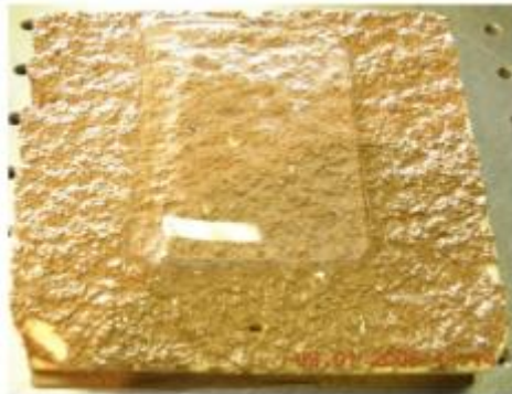
Protective coating for external fuel tank
